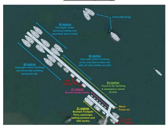
Figure one: Final overall design of the jetty.
