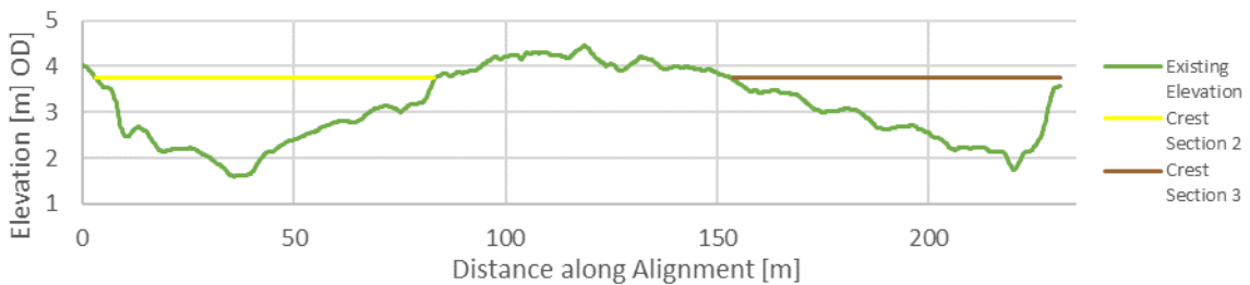
Figure 8-6 Cross section showing elevation and new embankment crest along Section 2 and Section 3 of the new embankment
